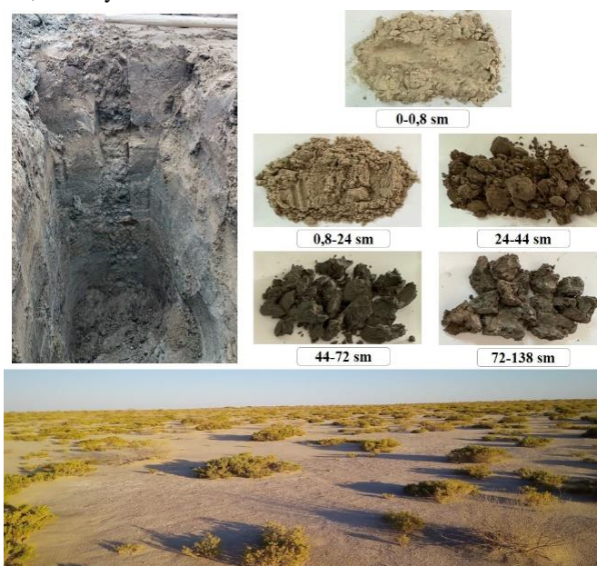
Fig. 7. Morphological features of profile 5 and soil samples on the dried-up bottom of the Aral Sea.
