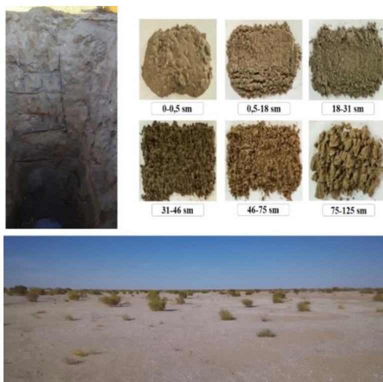
Fig. 5. Morphological features of profile 3 and soil samples on the dried-up bottom of the Aral Sea.
