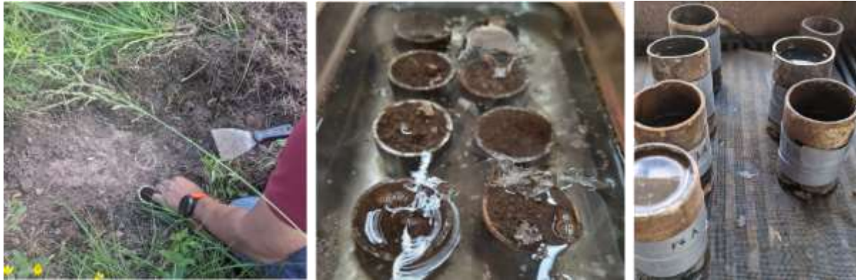
Fig. 4. Process for determining soil permeability.
