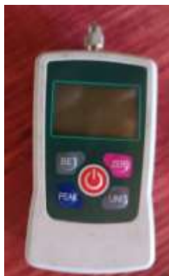
Fig. 3. Device for determining mechanical resistance to penetration.
