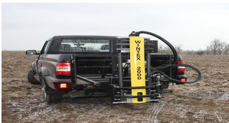
Fig. 3. Wintex Agro 2000 automated soil sampler for 0–20 cm sampling.
