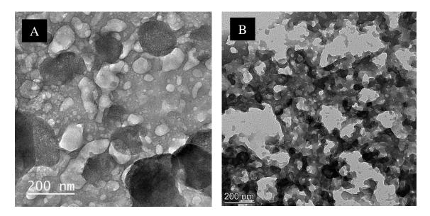
Fig. 3. TEM imaging of nano- NPK (A) and nano-micronutrients (B).
