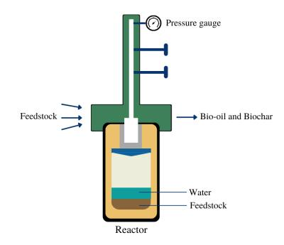
Fig. 5. Diagrammatic illustration of Hydrothermal Carbonization reactor (Du et al., 2019).
