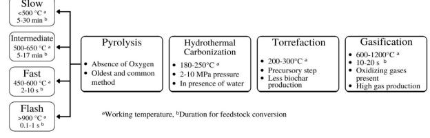
Fig. 1. Overview of production techniques of Biochar.
