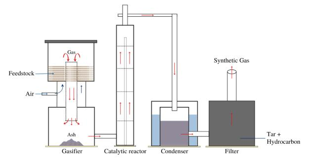
Fig. 6. Schematic illustration of the Gasification process (Dechapanya et al., 2020).
