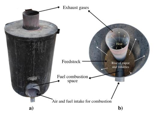
Fig. 4. Typical mobile domestic Pyrolysis stove, a) Front View, b) Top-Down View.
