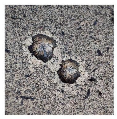
Fig. 7. Hydrophobicity showed by ground Rice-husk biochar.
