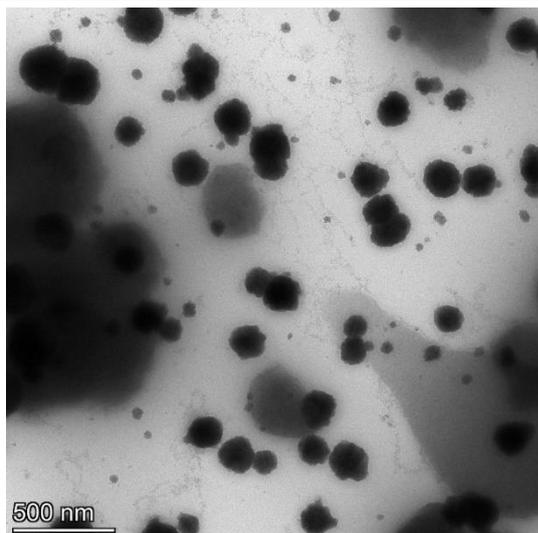
**Fig. 2. Transmission Electron Microscope (TEM) imaging of nano-sulfur.**
