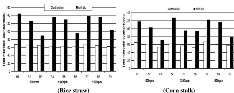
**Fig. 5. Effect of chopping machine rotation feeding rates and biofertilizers application on total microbial counts, of the matured compost for rice straw and corn stalk**
