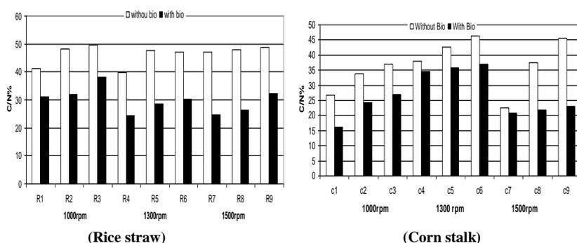
**Fig. 2. Effect of chopping machine rotation, feeding rates and biofertilizers application on C/N ratio, of the matured compost for rice straw and corn stalk**
