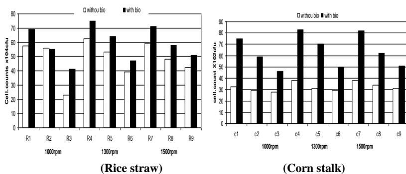
**Fig. 6. Effect of chopping machine rotation feeding rates and biofertilizers application on total microbial counts, of the matured compost for rice straw and corn stalk**
