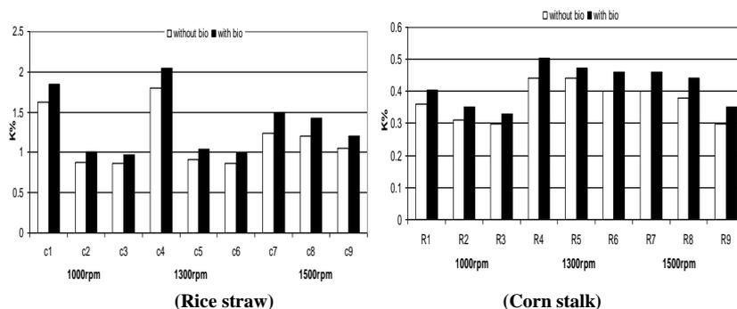
**Fig. 4. Effect of chopping machine rotation feeding rates and biofertilizers application on K%, of the matured compost for rice straw and corn stalk**
