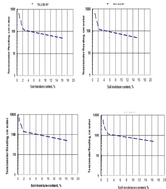
**Fig. 1 Relationship between soil moisture contents and Tensiometer reading under different saline waters in sandy soil.**
