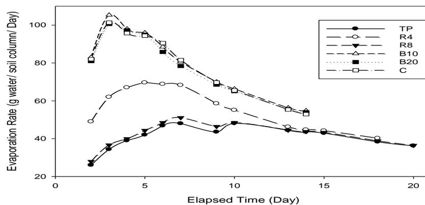
**Fig.1. Effect of different soil surface treatments on evaporation rate for Ismailia sandy soil during summer 2012**
