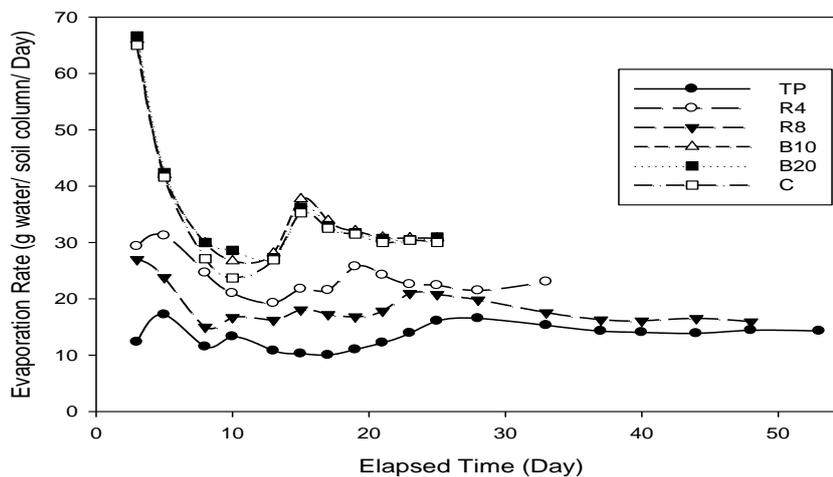
**Fig. 2.** Effect of different soil surface treatments on evaporation rate for Ismailia sandy soil during winter 2013
