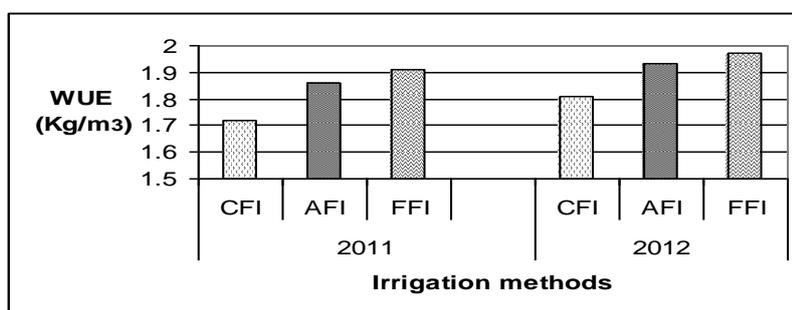
Fig.4. Water use efficiency (WUE) as affected by different irrigation methods.
